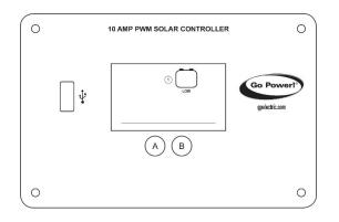
If the battery voltage reaches 11 volts, the battery SOC symbol will show the text "LOW" beneath it. The controller will continue operating in this condition and will only stop operating if the voltage drops below 9 volts.
