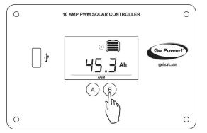
Push the **B Button** to show the number of amp hours charged since the last reset.
