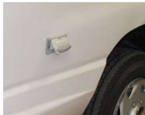
An external receptacle provides access to power from outside the vehicle, even with all doors securely closed.
