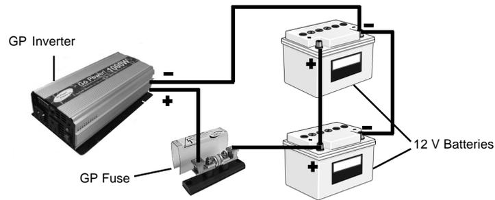
\*Installation using two 12 volt batteries.
