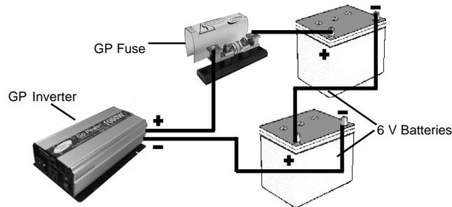
\*Installation using two 6 volt batteries.
